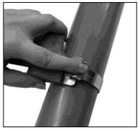
4. Place finger on BAND-IT Band at buckle bridge while tensioning with tool handle. When you feel BAND-IT Band stop moving through buckle as you are turning handle, *maximum pressure is being exerted by the BAND-IT Band* around object being clamped. *Stop turning handle.*
