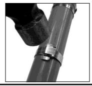
8. Hammer down buckle ears to hold band stub in place to complete BAND-IT clamp.
