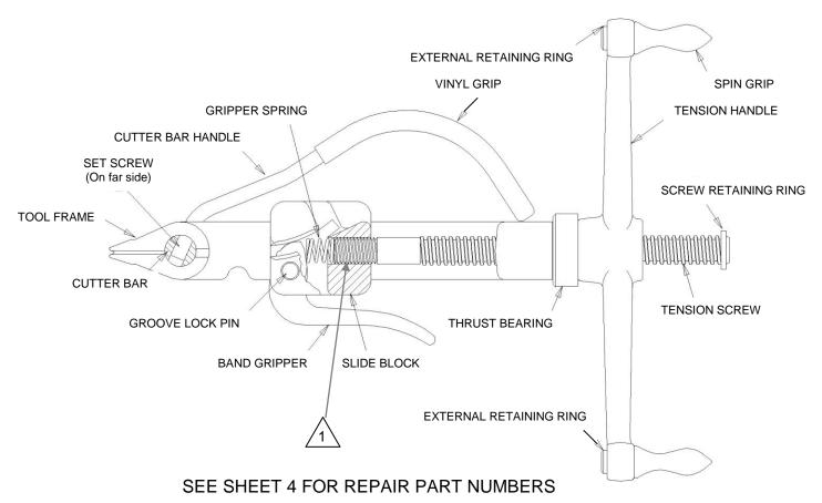
1. To assist in removing threaded parts, apply heat (softens locking compound).
