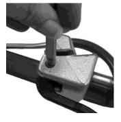
3. Replace pin. Gripper spring must be seated in tension screw hole. Align gripper hole with slide block hole, insert pin in hole and hammer pin in place.
