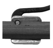
1. Remove gripper. Align gripper pin hole with notch in tool frame. Using a punch and hammer, punch pin out of slide block.
