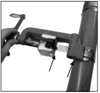
3. Place band in opening of tool nose and gripper block. Move into slot as far as possible, to avoid buckle sliding into tool nose. Tighten band clamp by turning the tension handle clockwise while holding band gripper tight against band. NOTE: The spring load of the band gripper is not intended to secure and prevent band from slipping during tension process.
